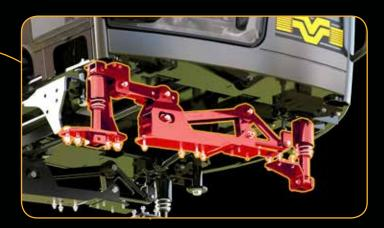
The suspended cab on the DeltaTrack (optional on the 4WD), combined with the optimization of the undercarriage provides the best ride in the industry.
